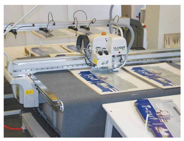
Material can be continuously retrieved from a roll of material, or sheets can be automatically fed through the Autofeeder sheet feeding system.
