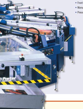
M&R's versatile Conquest multi-color UV print/cure system simultaneously prints and cures up to six colors.
