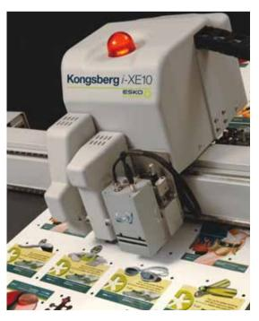
With the Kongsberg *i*-XE10 you can cut custom shapes right on the finishing table with exact registration between graphics and finishina.
