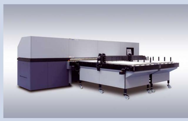
The Rho 900 is a 2.5m wide UV inkjet printer designed to offer the ultimate productivity combined with the finest quality print. It features automated media handling to maximise output and also additional process colours which extend the colour gamut.
