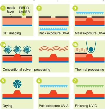
The digital flexo plate has a mask layer – sensitized to the CDI's laser light – on top of its surface. After imaging, this mask takes the function of the traditional film negative. Through the integration of the image carrier, a digital flexo plate has sharper image definition and steeper relief shoulders than conventional plates produced with film. Image deterioration by UV light absorption and scattering in the traditional contacting through vacuum sheet and film is totally eliminated.
