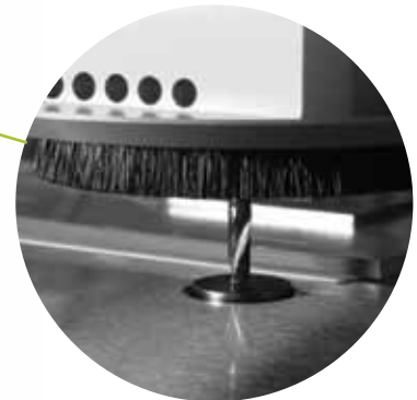
The Automatic Tool Leveling is a pressure sensitive pad that accurately and automatically calibrates the vertical operating level of all the Kongsberg XP tools.
